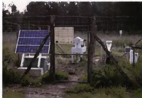
Weather station designed to measure atmospheric deposition in the Losse Forest in the Landes region (PM40c).
