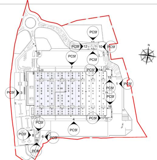
PLAN DE REPERAGE DES ELEVATIONS
